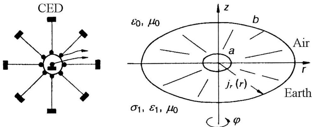
Figure 2. The “real” (left) and the “ideal” (right) circular electric dipoles comprising two concentric electrode systems discretely or continuously distributed along the circles of radius  $a$  (the inner or central electrode(s)) and  $b$  (the outer electrode(s)) respectively.
