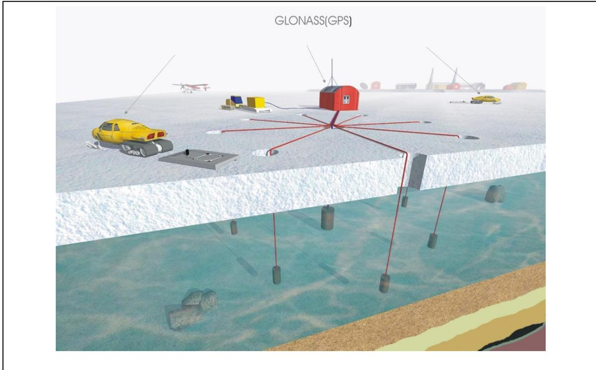
Figure 5. Layout of the CED transmitter in a drifting ice floe.
