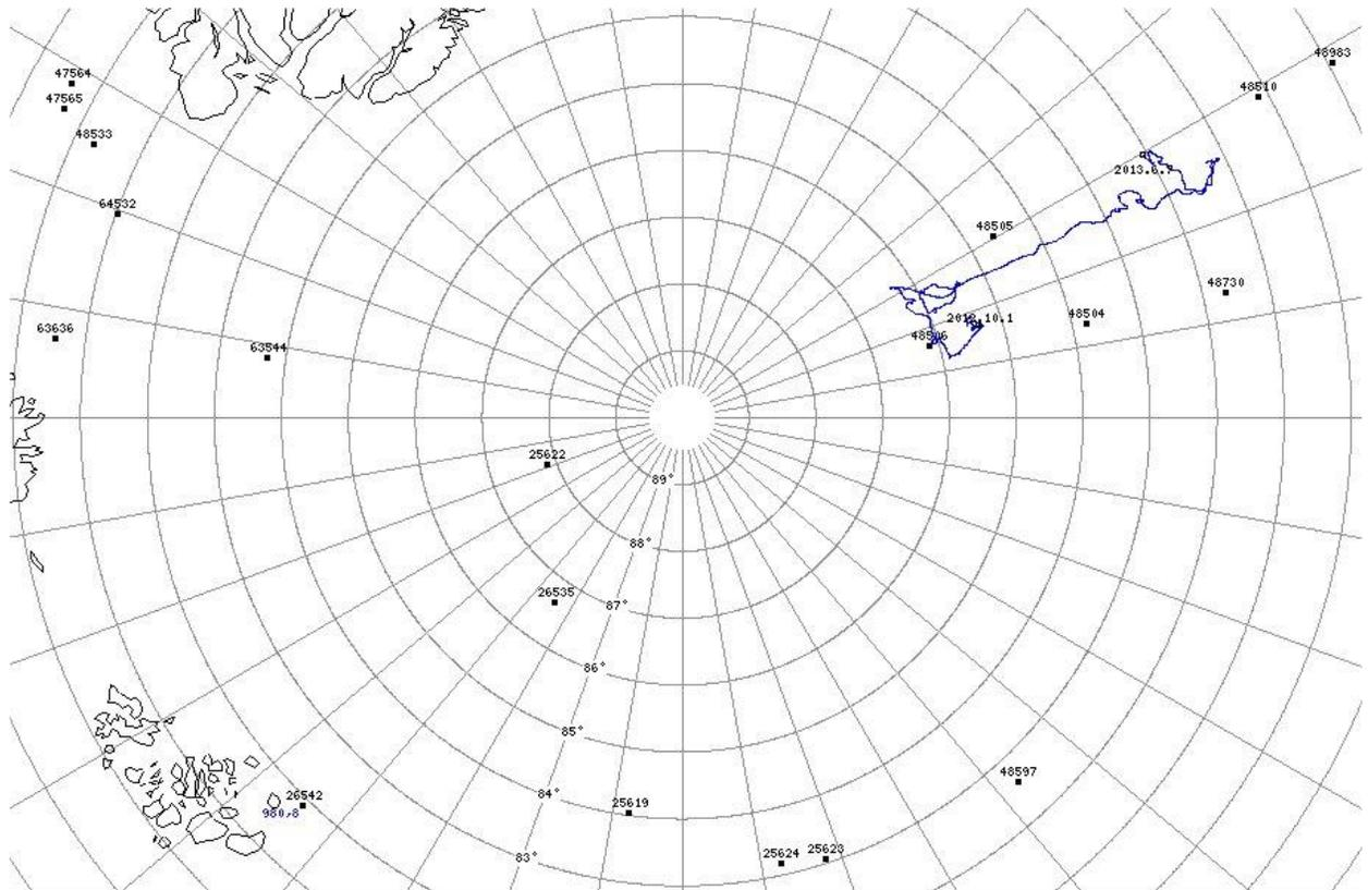
Figure 1. The travel path of the last polar station, NP-40, during the period from October 2012 to June 2013. A total length of the path is 1736 km.
